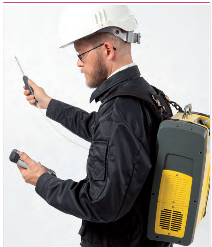
Using a portable FTIR gas analyser (Gaset Technologies model DX4040)
