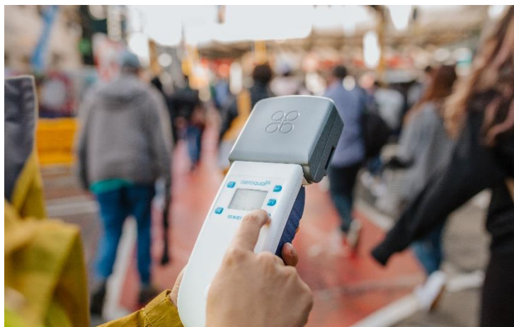
Small air sensors like this one can be used by anyone curious about local air quality. Photo credit: Aeroqual
