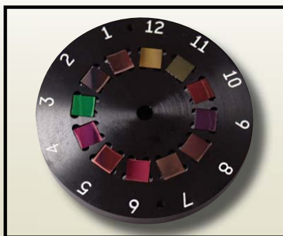
NDIR Optical Filter wheel directly measures NO 2
