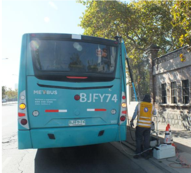
Figure 4: The emissions of solid particles from a bus in Santiago, Chile are measured to determine the condition of the DPF
